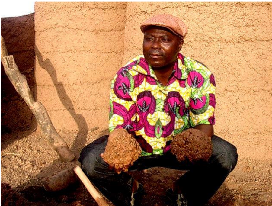
Figure 1: Picture showing mud balls ready to be used for construction in Koulangou, Togo. Yavo 2006.
